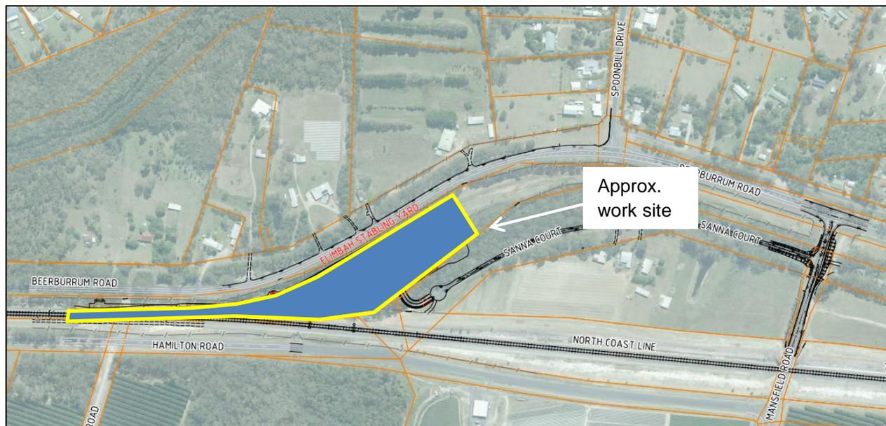
**Between midnight and 4am Tuesday 23 August 2016**, a track machine will be used to align the existing track to the turnout rail of the stabling facility. The track machine is used as part of Queensland Rail's normal maintenance program. It picks up section of track, compacts the ballast underneath and replaces the track into position.
