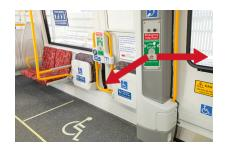
The emergency help button is close to train doors and allocated spaces.
