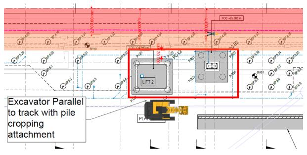
Figure 19 - SCA methodology Top View
