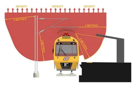
Figure 4 - Three (3) metre electrical exclusion zone - including pantograph
