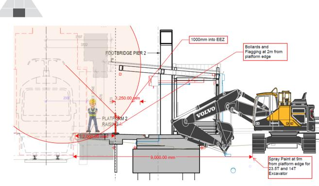
Figure 18 - SCA methodology Side View
