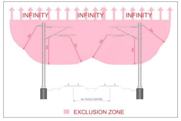
Figure 1 - Three (3) metre electrical exclusion zone
