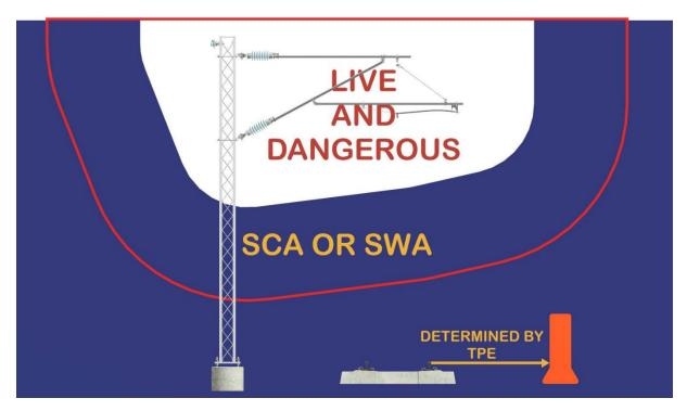
Figure 12 - Barrier distance approved by the Traction Power Engineer
