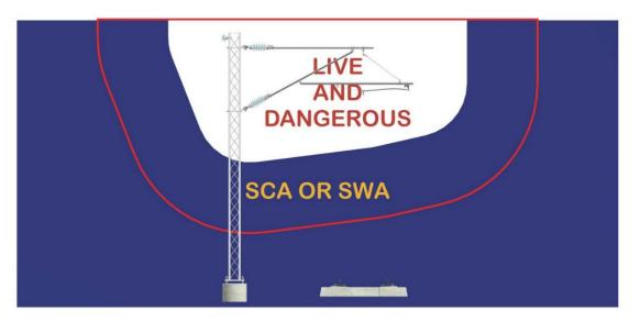
Figure 3 - Three (3) metre electrical exclusion zone - SCA/SWA
