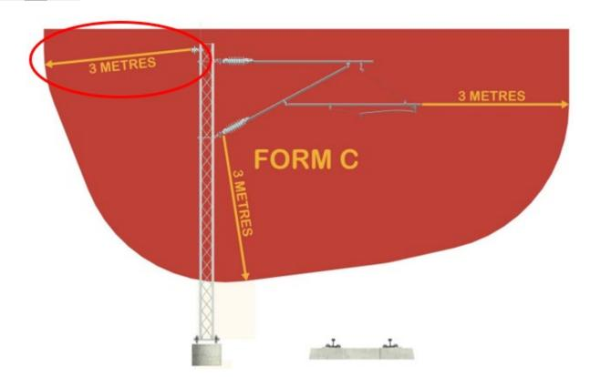
Figure 2 - Three (3) metre electrical exclusion zone - Form C
